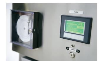
The main screen has both the alarm temperature and alarm set point(s) displayed. The alarm main screen flashes red and has an audible alarm which can be muted.
