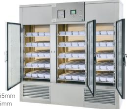
**Blood holding refrigerators** operate on R507 or R134a refrigerant. The cooling evaporator is fan forced with off cycle defrost and electronic alarm control that has a visual display of temperature.
